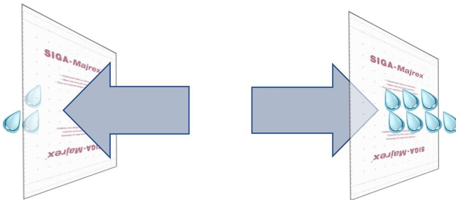
**Fig 7: Functional principle of directional smart vapor control layer SIGA MAJREX 200**
