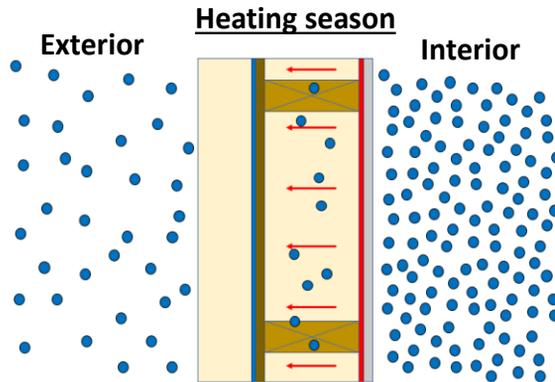
Fig 3: Direction of vapor drive during the heating season
