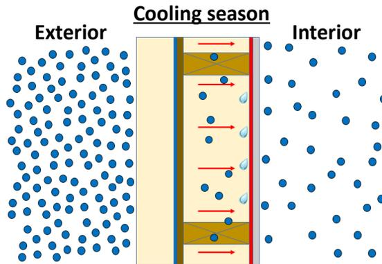
Fig 4: Direction of vapor drive during the cooling season
